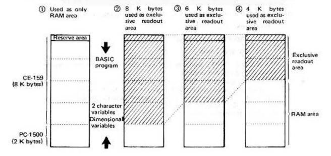
When the CE-159 is used as a RAM area, the reserve area can be secured inside the module, as illustrated. (The reserve area inside the PC-1500 can be cleared.) The BASIC program is written from the CE-159, while variables are secured from the PC-1500. With the CE-159 connected to the PC-1500, the total memory capacity becomes 10 K bytes including the reserve area.
