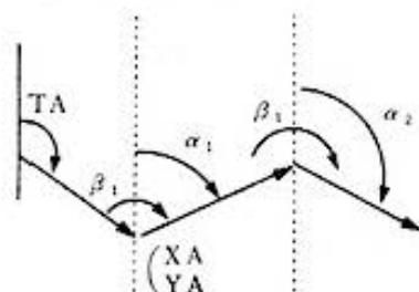
Azimuth  $\alpha_i = \alpha_{i+1} + \beta_i + 180^\circ - (360^\circ)$
