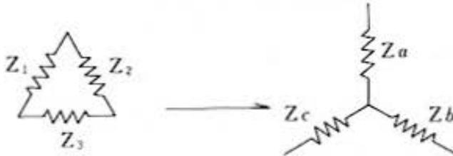
Also allows you to make an equivalent conversion from the impedance of Y connection to that of  $\Delta$  connection.
